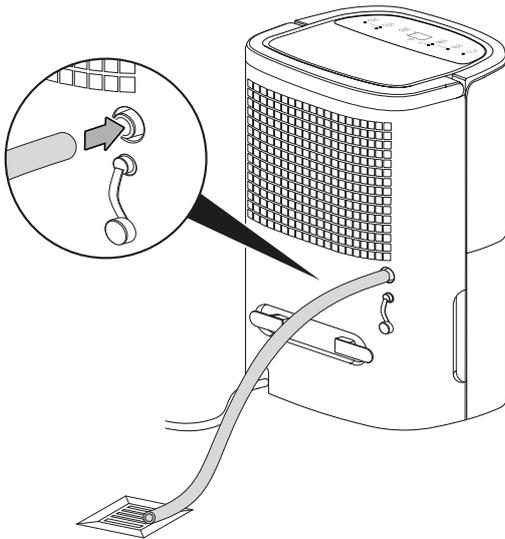
3. Guide the other hose end to a suitable drain or sufficiently dimensioned collection container. Please note that the hose must not be kinked.
