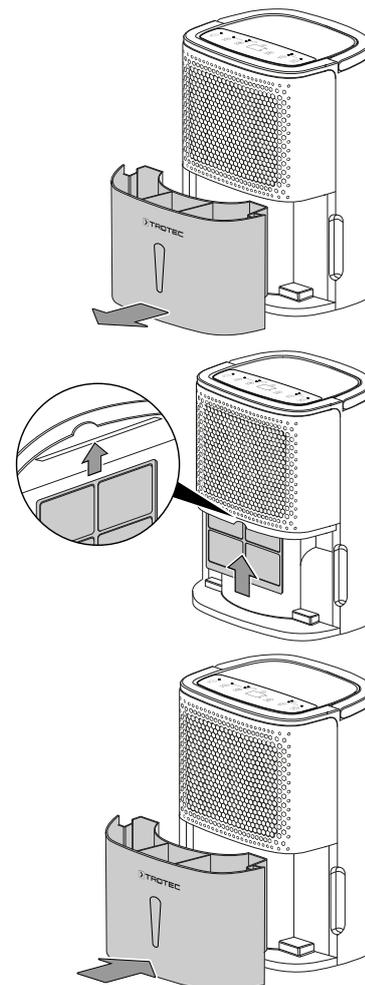
**Inserting the condensation tank**
