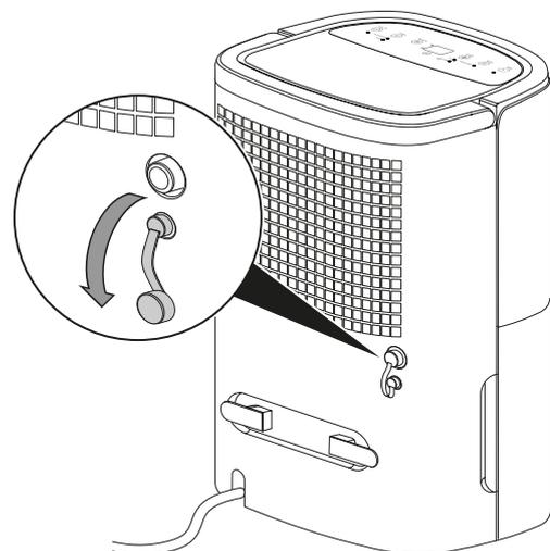
2. Push one end of the hose onto the hose connection.
